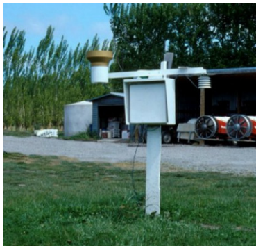
An electronic weather station linked to telephone modems and fitted with a range of sensors.
